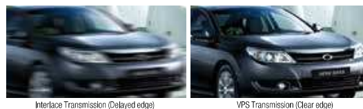
Interlace Transmission (Delayed edge)
